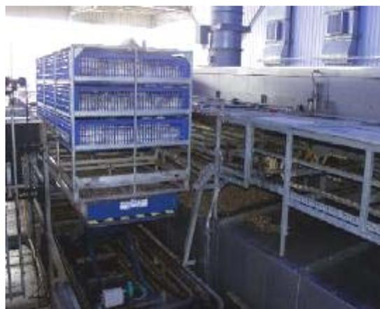
**Diagram 15: Crates being loaded into a controlled atmosphere stunner**
