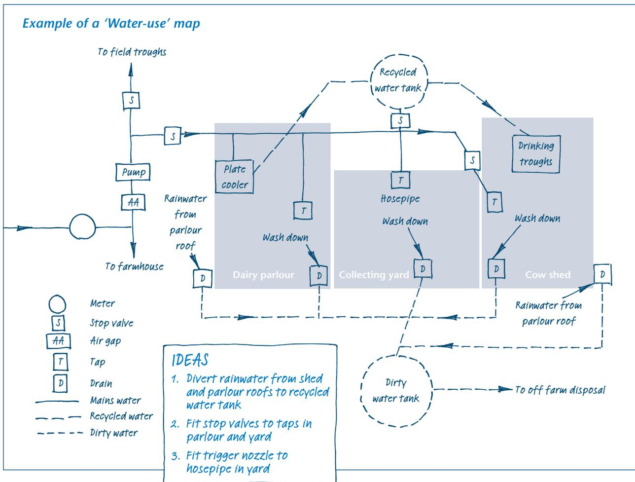
This map should indicate the location of all water uses, pipes, water troughs, taps, shut-off valves and stopcocks. You should also identify the sources of both clean and dirty water draining into the dirty-water system.
